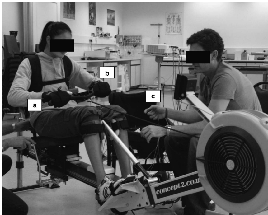
Figure 2 Equipment modifications to enable FES-rowing in tetraplegia. (a) Shoulder harness; (b) neoprene gloves; (c) attendant switching.
